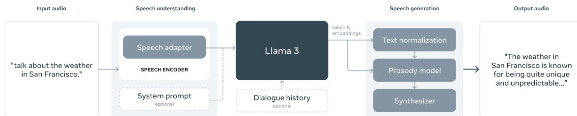
Figure 29 Architecture of our speech interface for Llama 3.
